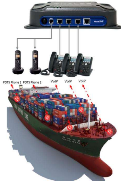
Figure 2-2 Local Communications via PBX Functionality
