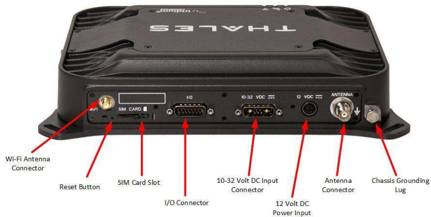
Figure 2-7 Below Deck Unit (BDU) Back Panel Detail
