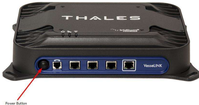
Figure 6-1 Location of Power Button on BDU
