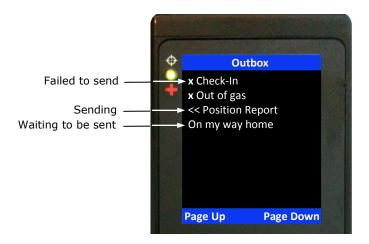
For each message queued in the Outbox, the nano attempts up to three times to transmit. After three failures, the message will be dequeued to avoid draining the battery. User has to manually requeue a message. If the nano is at a location not suited for transmission, user has to monitor the Outbox and repeatedly requeue until the message is successfully transmitted. The  $\triangle$  symbol appears on top of the home screen when there is a queued or dequeued message(s) in the Outbox.
