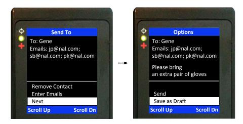
Once all required information is entered, user can either Send the message or Save as Draft. If Send is selected, a Success screen will appear to indicate that the message has been added to the Outbox. The nano must be held with the antennas having full view of the sky. If the Settings/Include GPS option is turned on then GPS location will be added to the message. Messages with GPS location takes longer to complete since the nano has to acquire a GPS fix.
