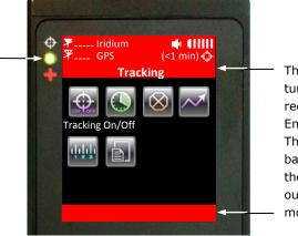
These two bars turn from blue to red under Emergency mode. They both turn back to blue when the device is taken out of Emergency mode.
