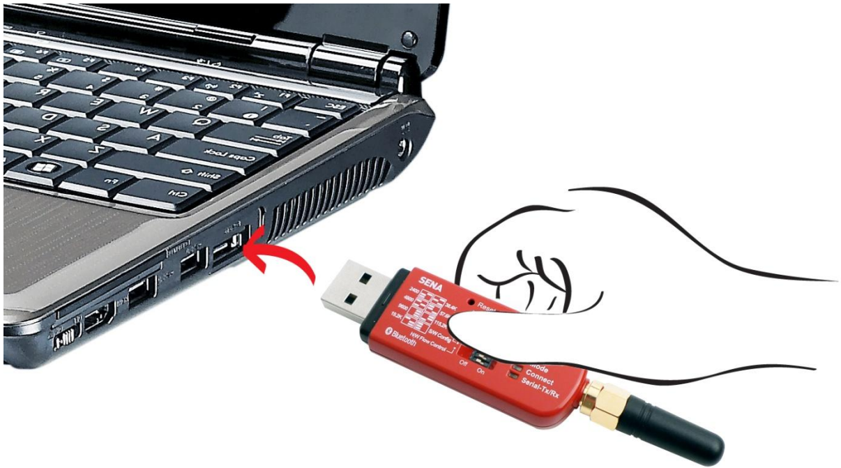
Figure 2-2 Connecting a Serial Device to Parani-SD1000U
