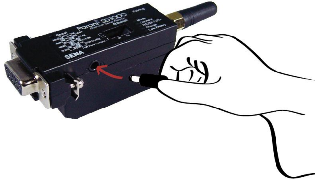
Figure 2-2 Connecting Power to Parani-SD1000
