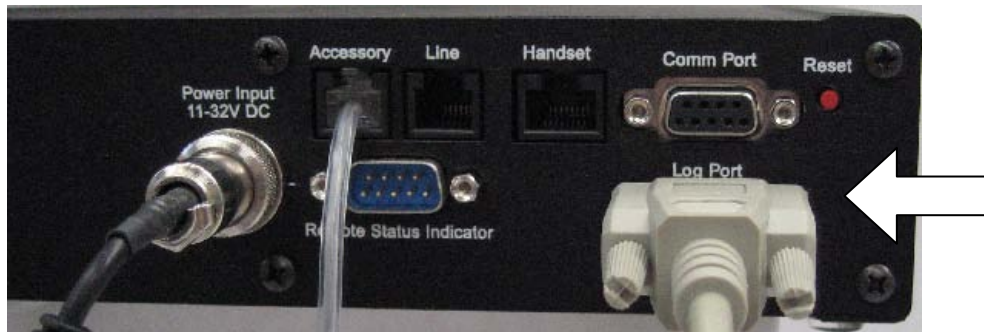
Figure: Serial cable connected to Log Port
