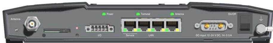
Figure 4-3: Service LAN connector used for configuration
