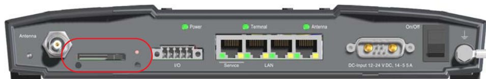
Figure 6-6: BDU connector panel
