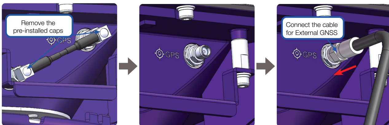
Figure 27: Connecting the SMA connector of the external GNSS cable to the GNSS connector
