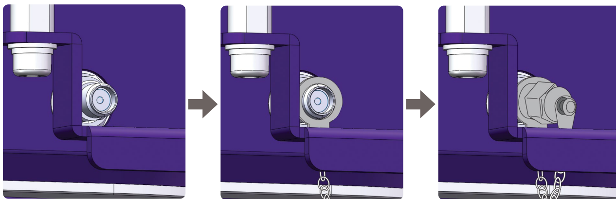
Figure 28: Close the left-hand connector (without GPS sticker) using the SMA cap provided
