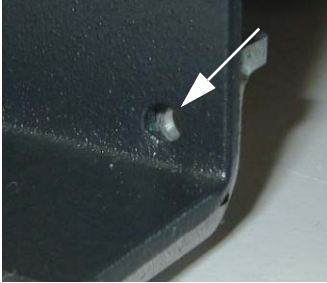
Figure 12: Holes for tampering seal
