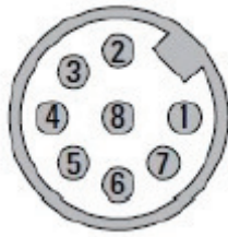
Figure 2-7 Connector Pin Positions
