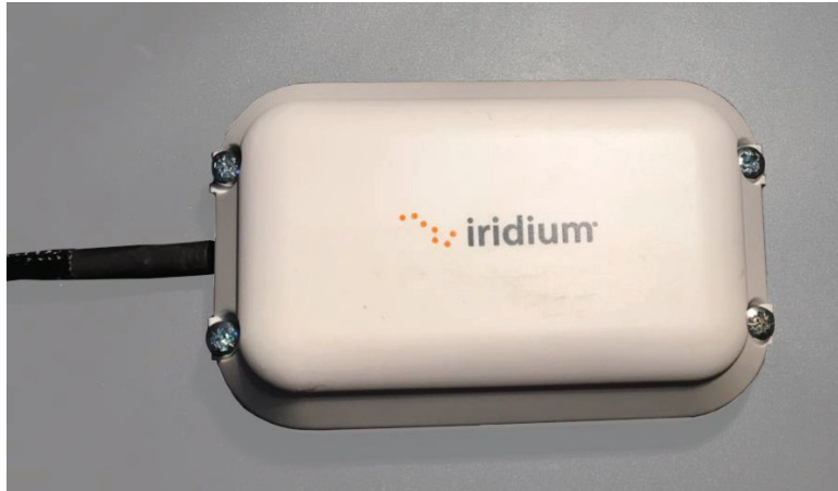
Figure 5-3 Screw Mount Installation
