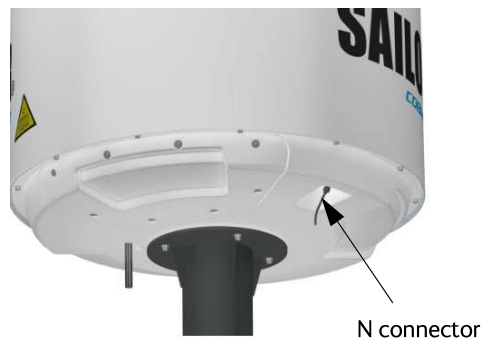
Figure 2-27: Connecting the ADU cable
