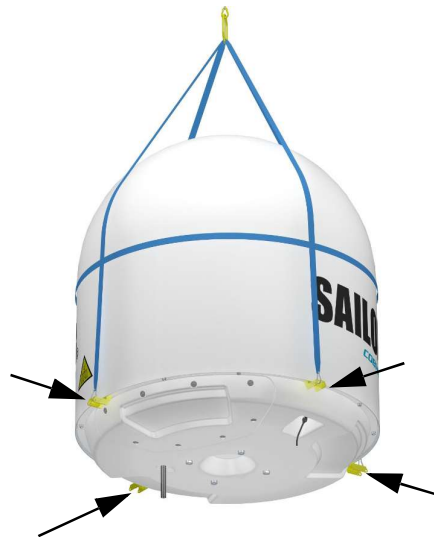
Figure 2-24: ADU installation, webbed sling attached to the 4 lifting brackets
