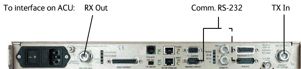
Figure C-14: Connecting COMTECH 570L to the ACU (example)
