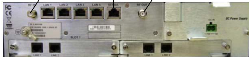
Figure C-20: Connecting Gilat SkyEdge II VSAT modem to the ACU
