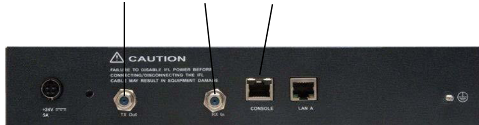
Figure C-11: Connecting iDirect Evolution X5 to the ACU (Serial)
