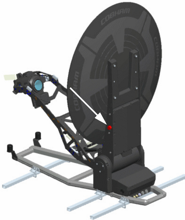
Figure 4-7: Emergency stop button
