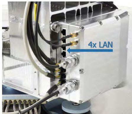
Figure 2-21: ACM LAN ports
