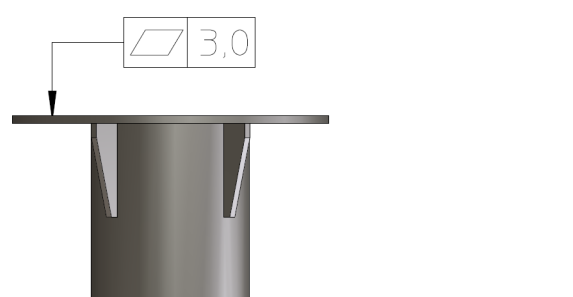
Figure 2-9: ADU mast flange, recommended flatness on the mast mount plateau
