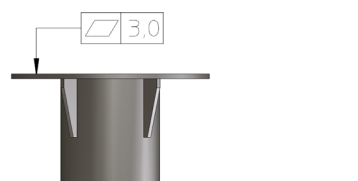
Figure 2-5: ADU mast flange, recommended flatness on the mast mount plateau
