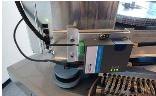
Figure 2-38: LTE modem connection, example
