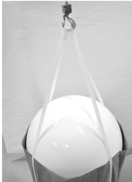
Figure 2-28: ADU installation, 4 lifting straps on crane hook
