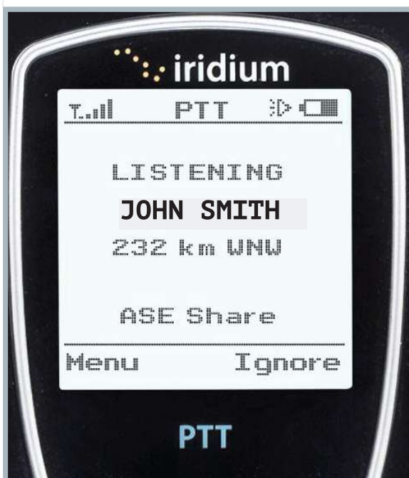
WITH GPS ANTENNA-POSITION KNOWN
