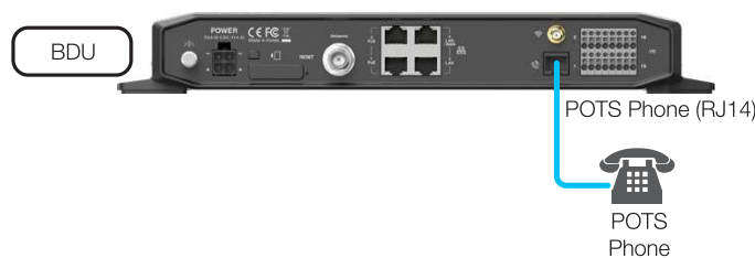
Figure 34: BDU to POTS Phone (RJ14) Cable Connection
