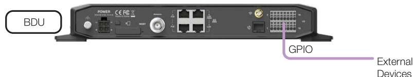
Figure 36: BDU to External Devices Connection
