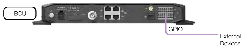
Figure 41: BDU to External Devices Connection
