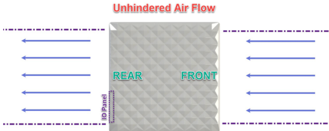
Figure 7: Airflow path required to support passive cooling.
